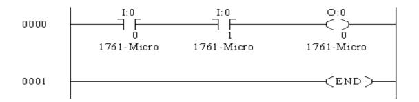
Thus the actuation of single acting cylinder with and AND gate was done.
