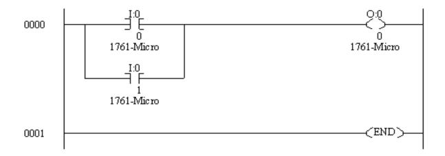
Thus the actuation of single acting cylinder with and OR gate was done using PLC.
