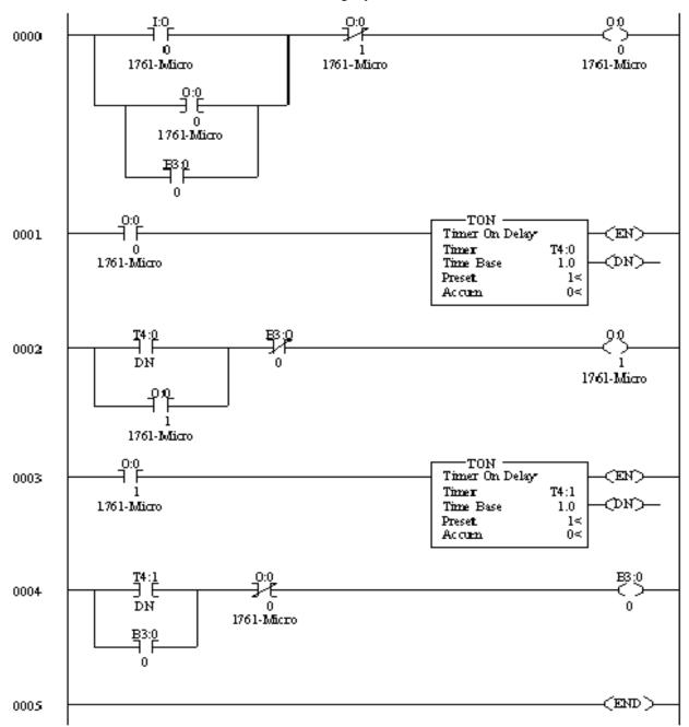
CIRCUIT (Automatic Actuation Of Double Acting Cylinder)
