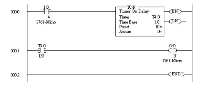
Thus the actuation of single acting cylinder with ON Delay timer was done using PLC.
